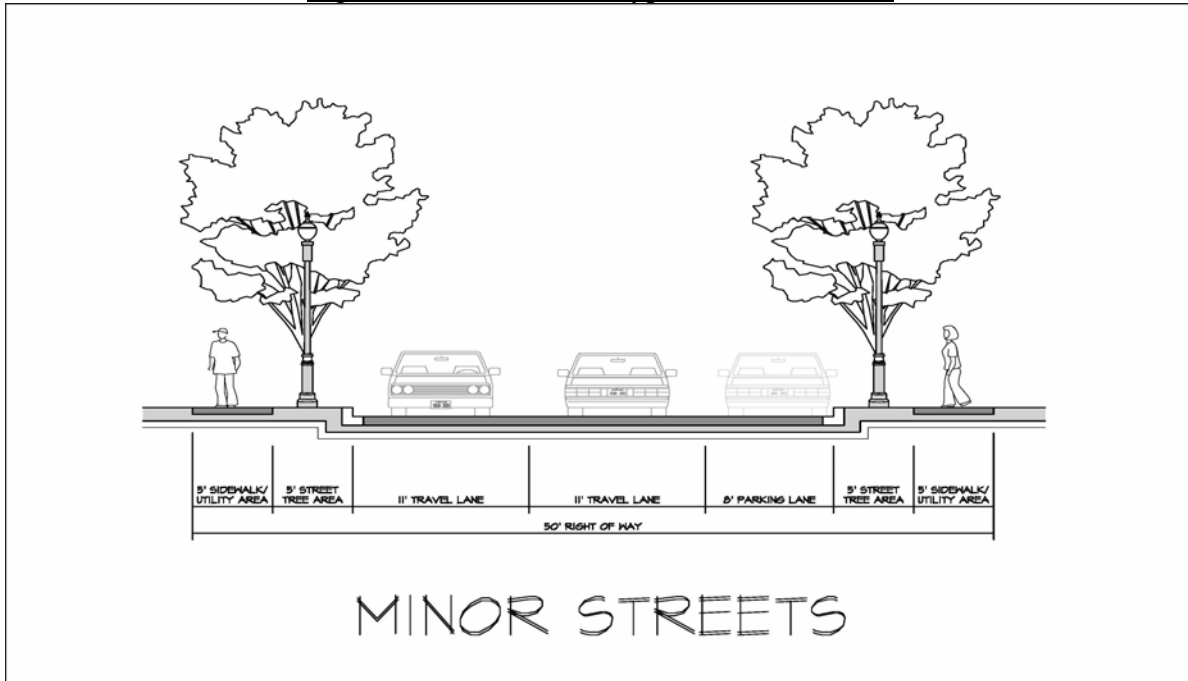
Figure 1: Minor Street Typical Cross Section
