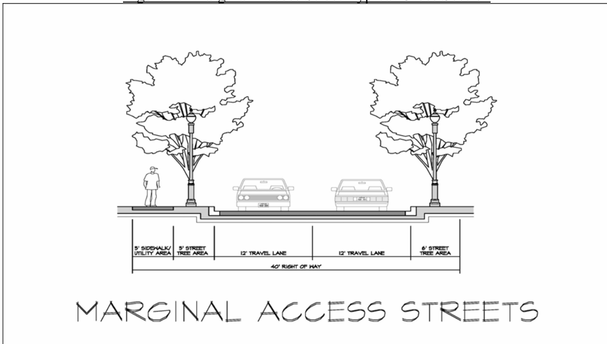
Figure 2: Marginal Access Street Typical Cross Section
