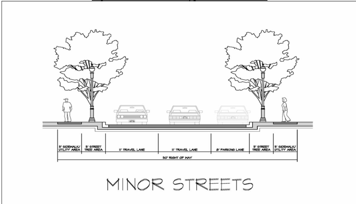
Figure 1: Minor Street Typical Cross Section
